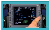
ACARS is a system enabling an exchange of simple text messages between the pilot and the controller
